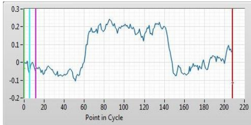
PMT signal per one cycle – “optical curve”
